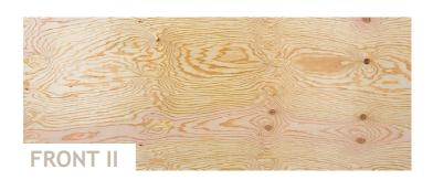
Closed face, with sound knots and wood patches Ad hoc sealant repairs
