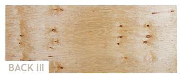
Open face, not repaired, possibly with holes, knots and cracks
