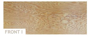
Closed face, without knots and with wood patches (max 5/m<sup>2</sup>). Ad hoc sealant repairs
