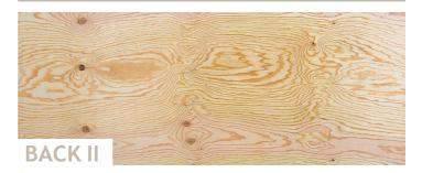
Closed side, with sound knots and wood patches Ad hoc sealant repairs
