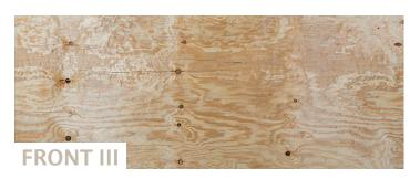
Face not repaired, possibly with knotholes and cracks
